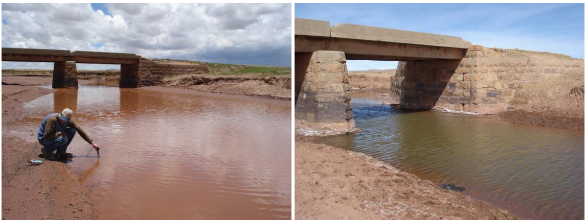
Figure 15. The photo on the left is RK-2 during the January 2009 sampling event, and the photo on the right is from the June 2009 sampling event. The amount of flow and suspended sediment decreased between the two events. In June 2009 there was precipitates present on the bank of the river and algae in the river.
