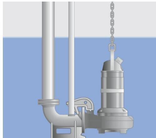
*Examples of submersible sewage pumps that could be used at Calauma's Rehab Center to move sewage via pressure force main (via 2" or 3" pvc or hdpe) uphill 1.3 km to Viacha's nearest manhole.*
