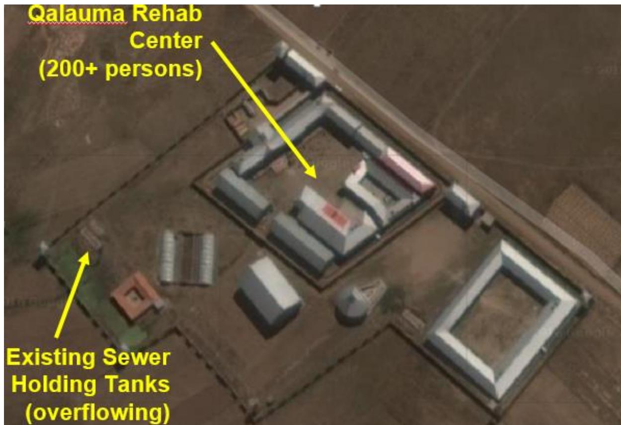
The wastewater from the facility is piped to the northwest corner inside the fenced facility, to a couple concrete holding tanks which are completely full, resulting in ponding of contaminated water in various
