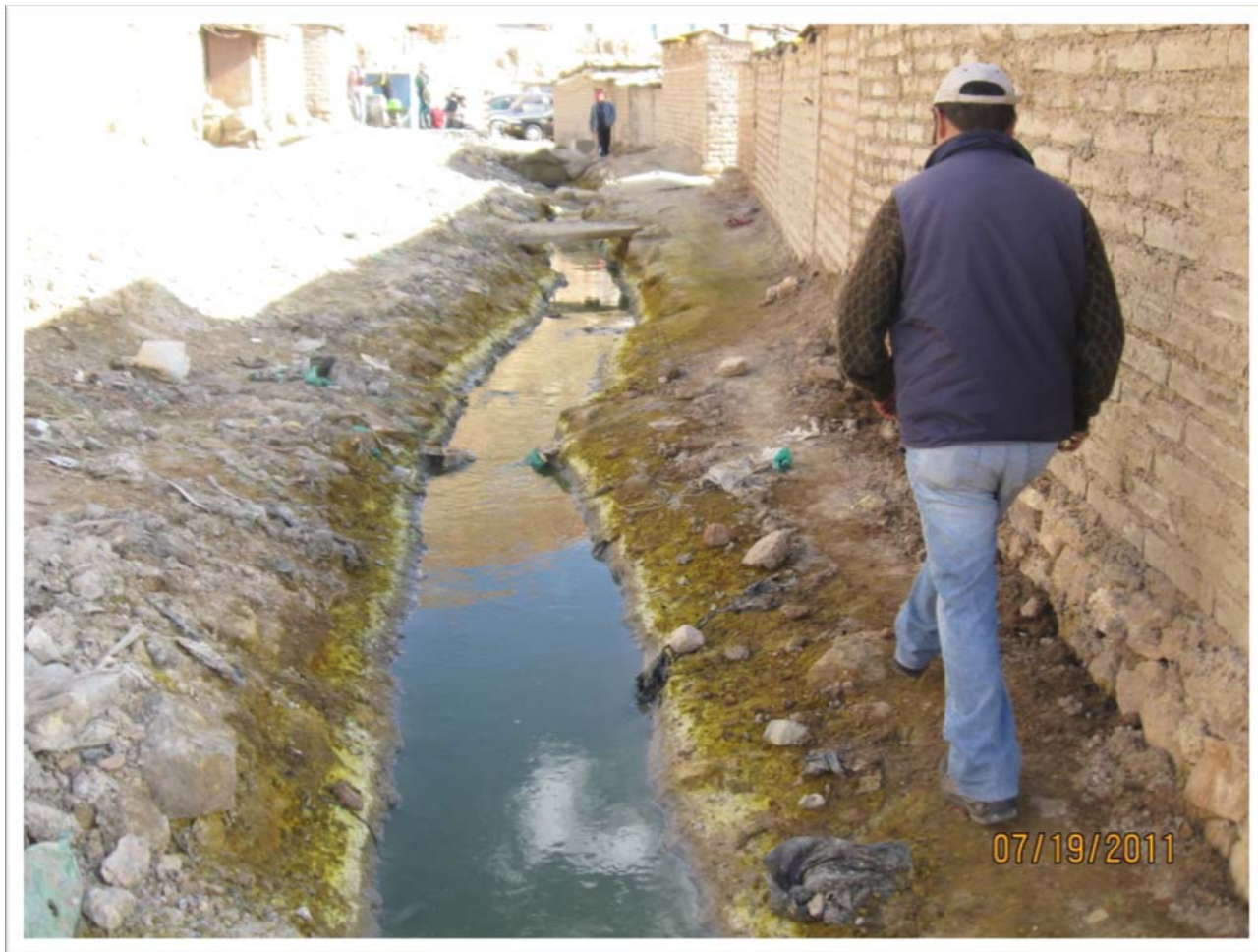
Figure 7 - Drainage from San Jose Mine, yellow material is elemental sulfur precipitated from pH 1 water
