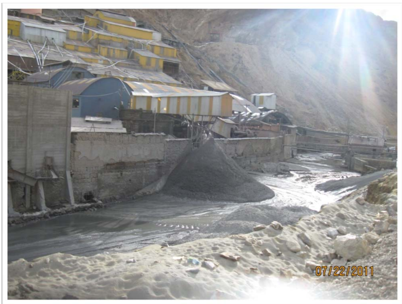
Figure 1 – Santa Elena Mill with tailings deposited in Huanuni River at Posokoni Mine
