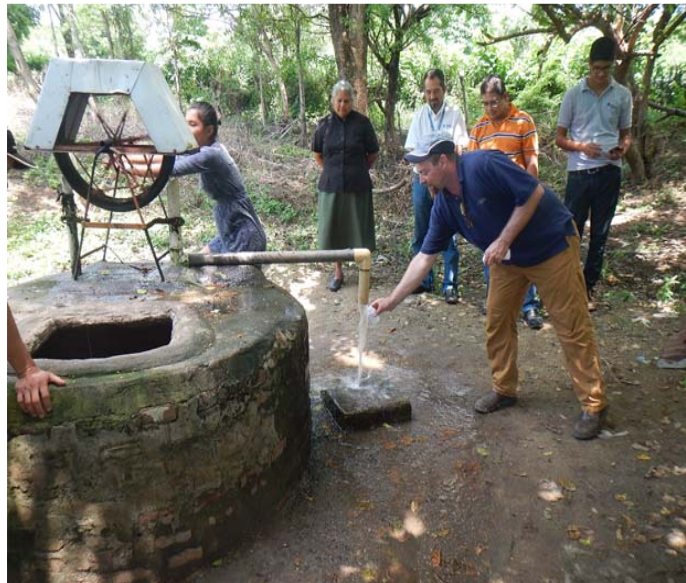
Scott McKitrick collecting a water sample from a hand-dug well in Tepeagua for later analysis
