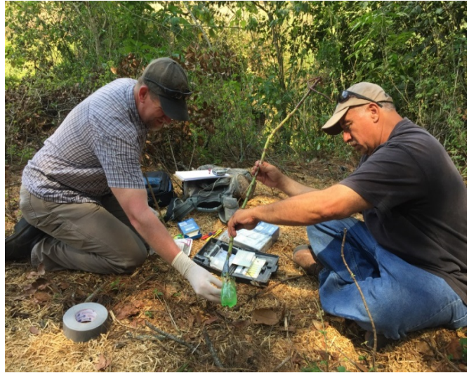
Ewan and Marvin conduct ammonia and nitrogen tests of the river water downstream of the existing sewage discharge point, to assess the impact on the river from the existing system.
