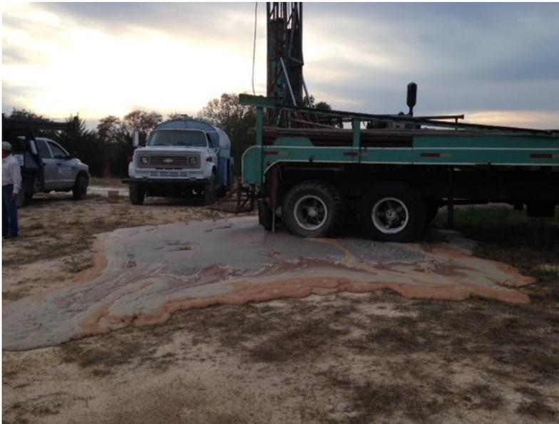
*During Braulio's visit to Texas and New Mexico in mid-October, he was introduced to foam drilling by Dale White, shown here. Dale explained the stops that would be needed if desired by Suma Jayma to retrofit their own drilling rig to be able to use compressed air/foaming agent in lieu of drilling mud with bentonite.*
