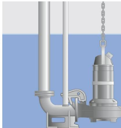
*Examples of submersible sewage pumps that could be used at Calauuma's Rehab Center to move sewage via pressure force main (via 2" or 3" pvc or hdpe) uphill 1.3 km to Viacha's nearest manhole.*
