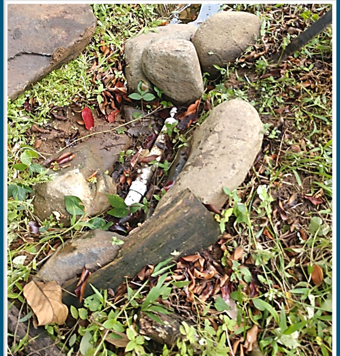
Running a transmission line down steep grades causes the joint to pull apart if not anchored properly. One area with multiple repairs.
