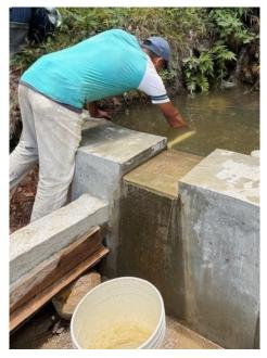
Then we measured flow coming out of the transmission line. It was only 2 gpm. So we hiked up to the spring and found it was overflowing around 14 gpm. This was a relief; it meant the problem was in the pipeline and not that the spring had dried up. After walking the line, we determined the problem was debris or sediment buildup in a low section just below a cliff. We will fix this by installing a clean-out valve at this location, using one of the left-over 1.5" gate valves.
