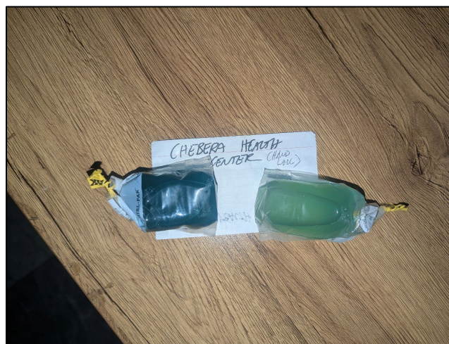
Figure 15: Blue-Green color of Chebera water samples indicating presence of E. Coli and Total Coliform
