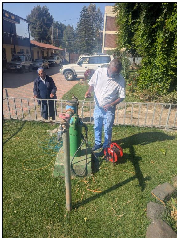
Figure 22: Dr. Tilahun measuring the Depth to Water while Sister Aster watches closely.
