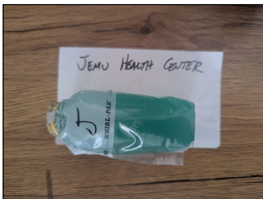
Figure 12: Blue-Green color of the Jomu water sample indicating the presence of E. Coli and Total Coliform
