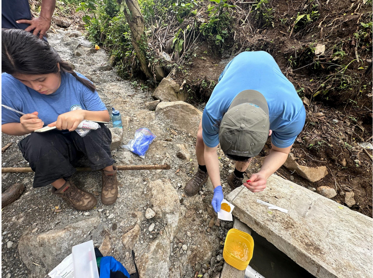
Figure 1: Rapid E.Coli/coliform and nitrate/nitrite testing at Mario Lopez 2 intake
